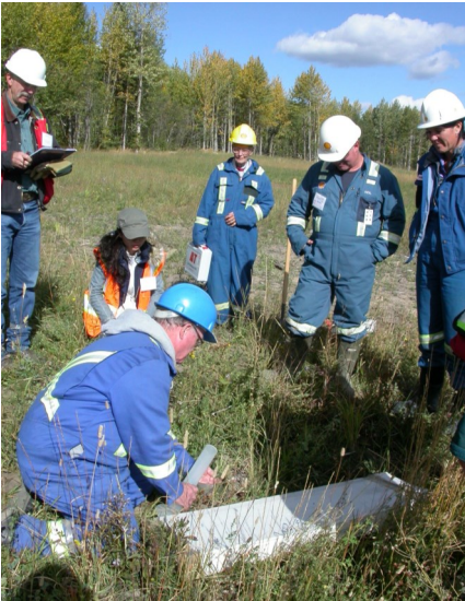
Bill McGill demonstrates how to measure water infiltration and soil moisture (photos left & above). He shows Kristin Kendrew how to measure soil compaction and take bulk density samples (right).
