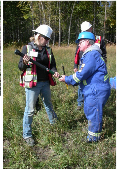
Bill McGill demonstrates how to measure water infiltration and soil moisture (photos left & above). He shows Kristin Kendrew how to measure soil compaction and take bulk density samples (right).
