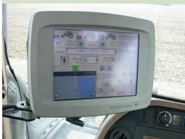
Monitor in Rod’s tractor to set & monitor variable rates of fertilizer during seeding.
