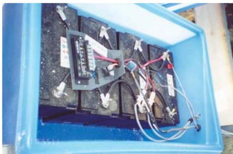
Four 12 volt batteries hooked in parallel
