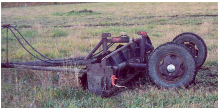
The "Cowger modified" blade worked well for spreading manure evenly over the pasture.
