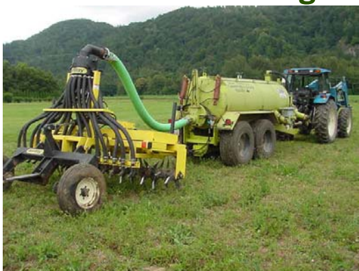
Injecting manure with AerWay Sub-surface Deposition equipment in the Lower Mainland.
