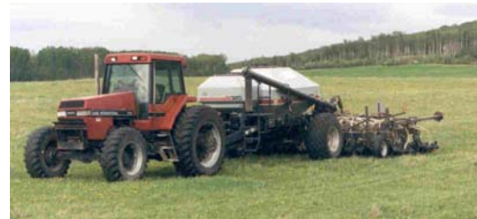
The Flexicoil zero till drill with Barton openers, fertilizing and seeding at Peter Van Genne's plot.
