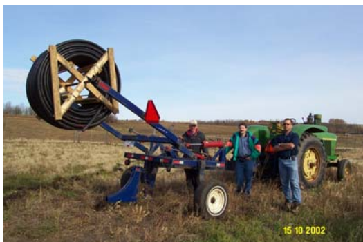
Pasture Pipeline Plow was used at Bill Wilsons to put in pipe for remote water access.
